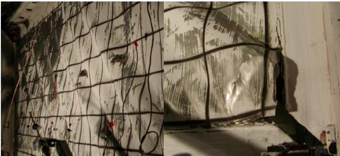
Figure 3 Light-Gauge SPSW Hystereses – Infill Only (Berman and Bruneau, 2003b)
