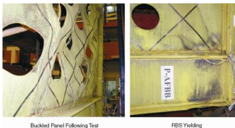
Figure 6 Buckled Panel and RBS Yielding of SPW Specimen (Vian and Bruneau, 2004)
