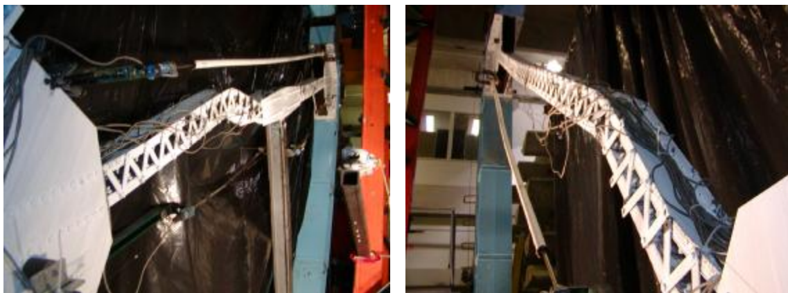
Figure 14 Global buckled shape of various specimens (Lee and Bruneau, 2004)
