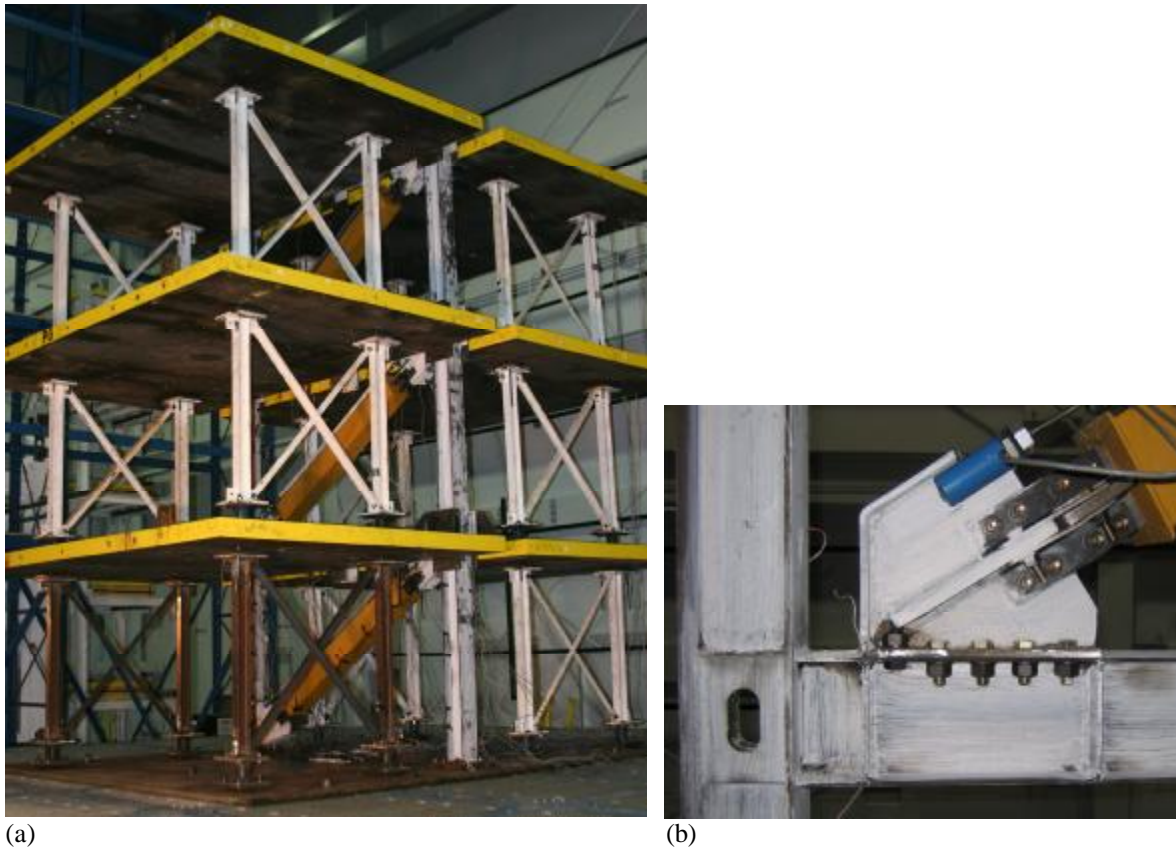
Figure 11 (a) Three-story Shake-Table Test Specimen; (b) removable and eccentric gusset plates (Vargas and Bruneau, 2006b)
